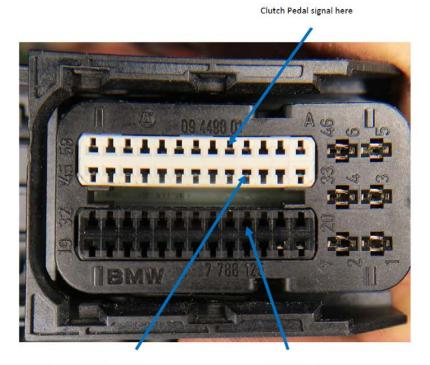
Brake Pedal signal 1 here
