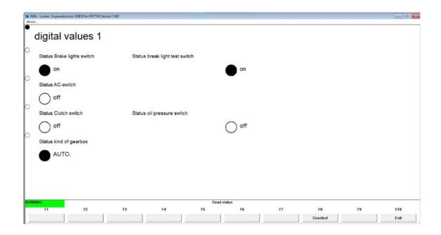
Please also verify the gearbox type as shown at the bottom of the screen. If your ECU is configured for the wrong type, it will not work! Please send your ECU to be reconfigured to the correct gearbox type if this is the case.
