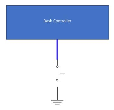
Fuel pump relay trigger: Some looms that are currently available for purchase will already have this option (e.g. House of Torque). You can use either output. The switched earth output in the dash controller will run the pump for 10 seconds with the ignition on, then go off. It will restart when you crank the engine over. Below is a diagram showing how you should connect the fuel pump relay:
