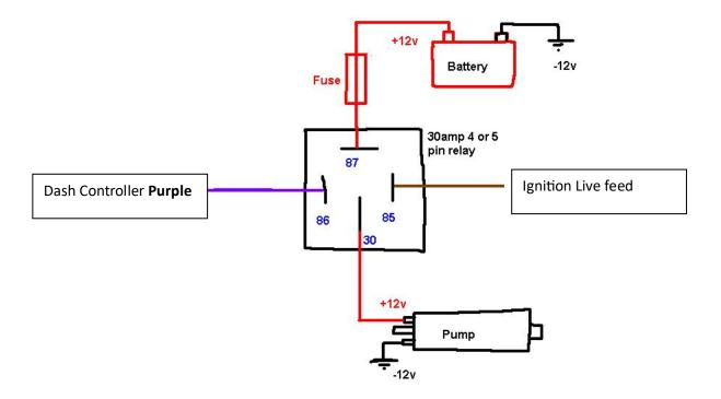
Note: The dash controller will also active the standard Transit MK8 lift pump in the tank. If it not required you can simply remove the relay for the fuel pump, located in the engine bay fuse box.
